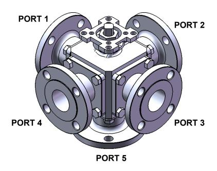
EXAMPLE: A SERIES 53 (5-WAY) VALVE SPECIFIED WITH A "TT" PORT AND "U" ARRANGEMENT IN BALL POSITION "1" WILL HAVE FLOW PATHS OPEN AT PORTS 1,3, 4, AND 5.
