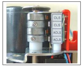
Rotate the OLS cam CCW towards the limit switch lever until the switch 'clicks'. Tighten setscrew with allen key.
