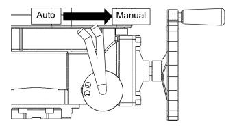
Actuator rotation direction is cast on the handwheel. Rotating handwheel in the identified direction will rotate the actuator output as follows.
