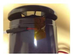
The red tip of the Thermistor must touch the outside of the motor housing. We recommend using high temperature tape to hold the tip to the surface.
