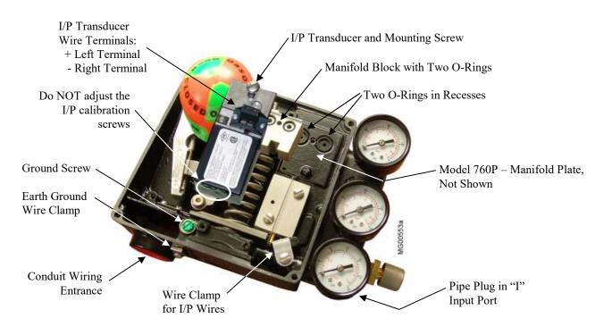
Figure 4-11 I/P Installation, Exploded View
