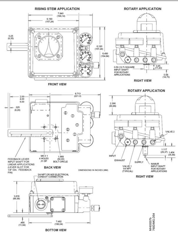
Figure 2-1 Installation Dimensions, Design Levels A and B
