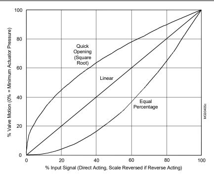
Figure 3-3 Standard Cam Characteristics
