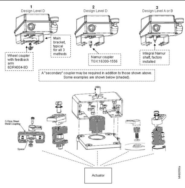
Figure 2-14 Rotary Actuator, Basic Feedback Methods
