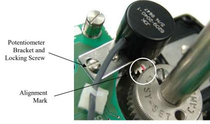
Figure 4-5 Potentiometer Alignment
