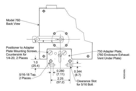
Figure 4-13 Model 760 Positioner with Optional Model 750 Adapter Plate
