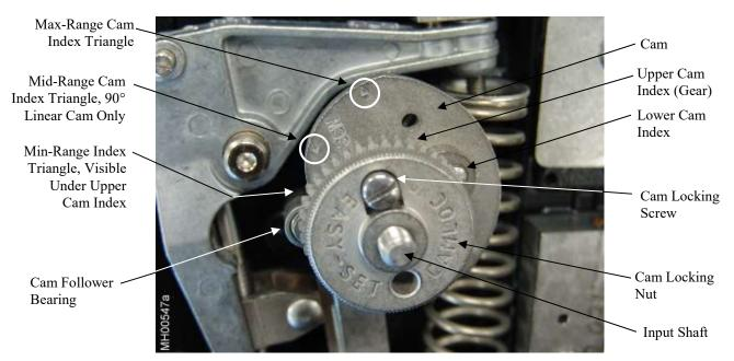
Figure 3-1 Cam and Cam Indexing Components
