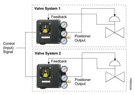
As an example, in the above figure, Valve System 1 operates from the fully closed position to its fully open position when the control signal goes from 4 mA to 12 mA (or 3 psig to 9 psig). Valve System 2 remains closed during this first portion of the control range, opening only when the control signal reaches 12 mA (or 9 psig). It continues to open to its full position when the control signal reaches 20 mA (or 15 psig). Reverse action is also possible on one or both of these devices.
