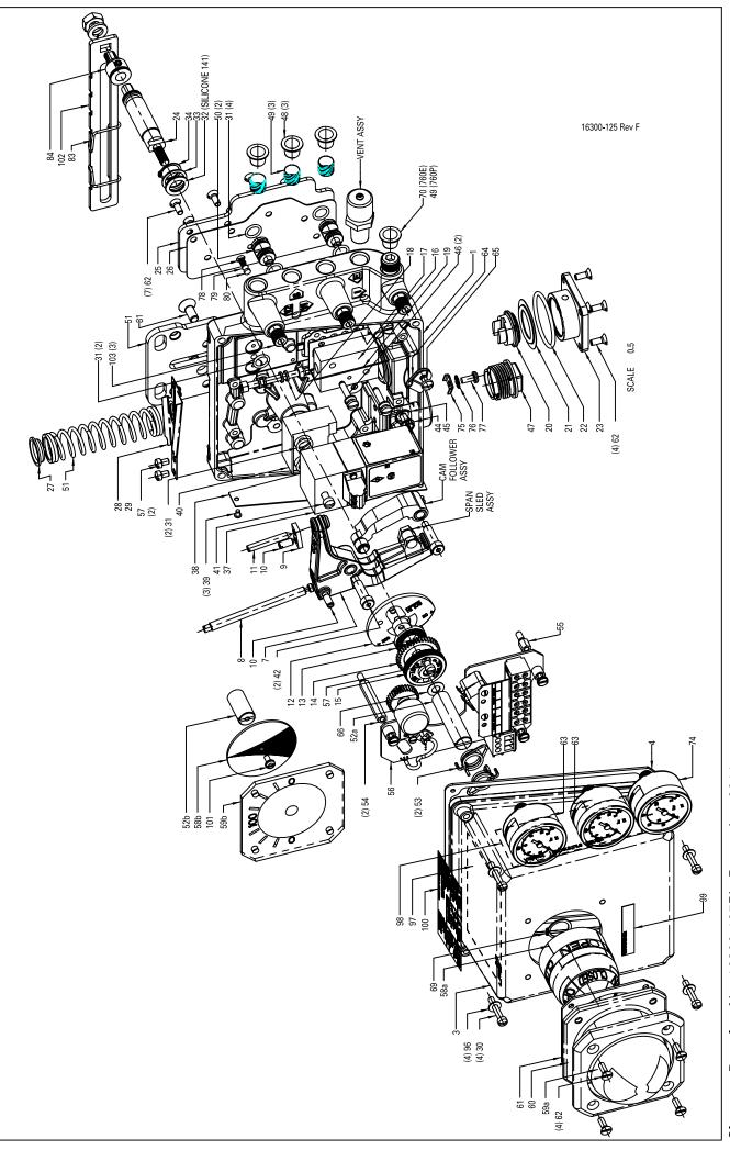
Series 760 Valve Controller Exploded View, Design Level "D"
