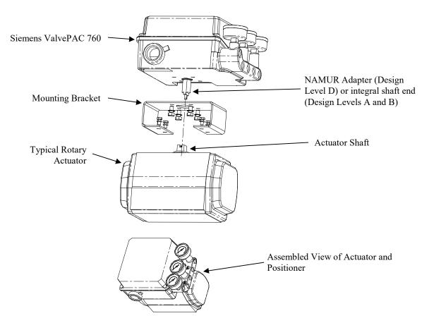
Figure 2-12 Positioner with Rotary Actuator Example
