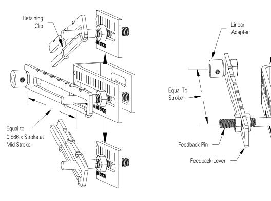
B. Preferred Method of Stroke Setting for Feedback Pin Connection
