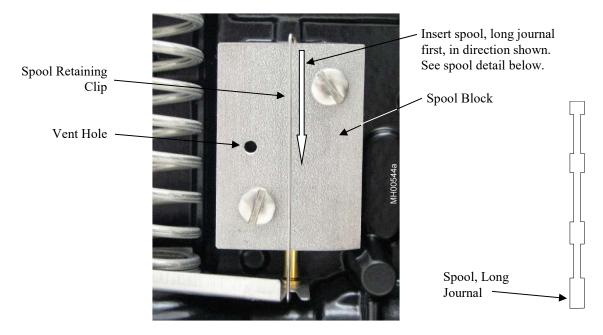
Figure 4-12 Output Capacity Spool Kit
