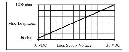
Figure 4-7 Maximum Loop Load vs. Loop Supply Voltage
