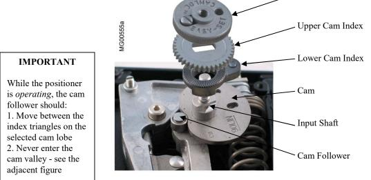
Figure 3-4 Cam Index Components
