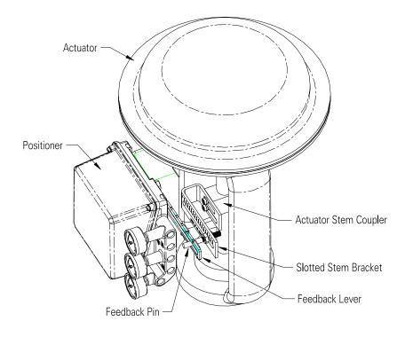
A. Positioner Mounting and Preferred Method of Connecting Feedback Pin
