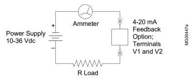
Figure 4-6 4-20 mA Loop Calibration
