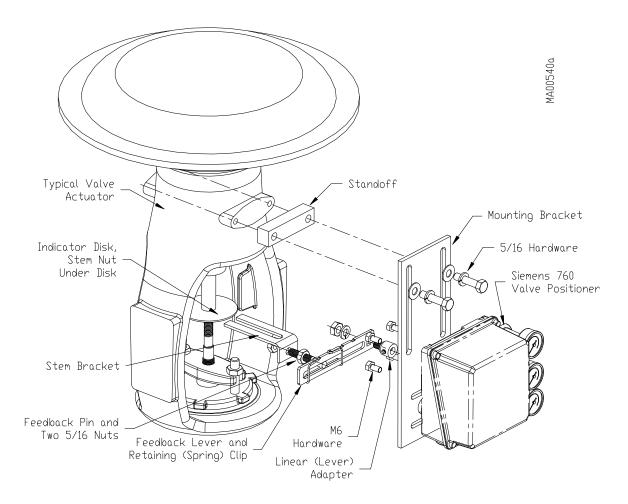
Figure 2-4 Positioner with Typical Linear Actuator
