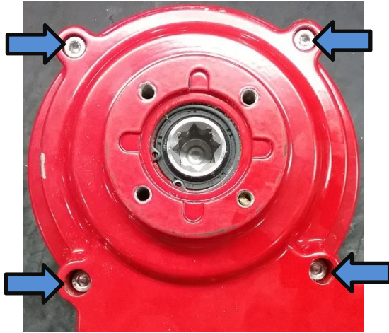
FSE/FSEM gear override actuator mounting plate bolts.
