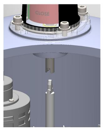
Lower the body cover onto the body until the contact surfaces are mated together. Make sure that bolt holes and indicator are aligned properly.
