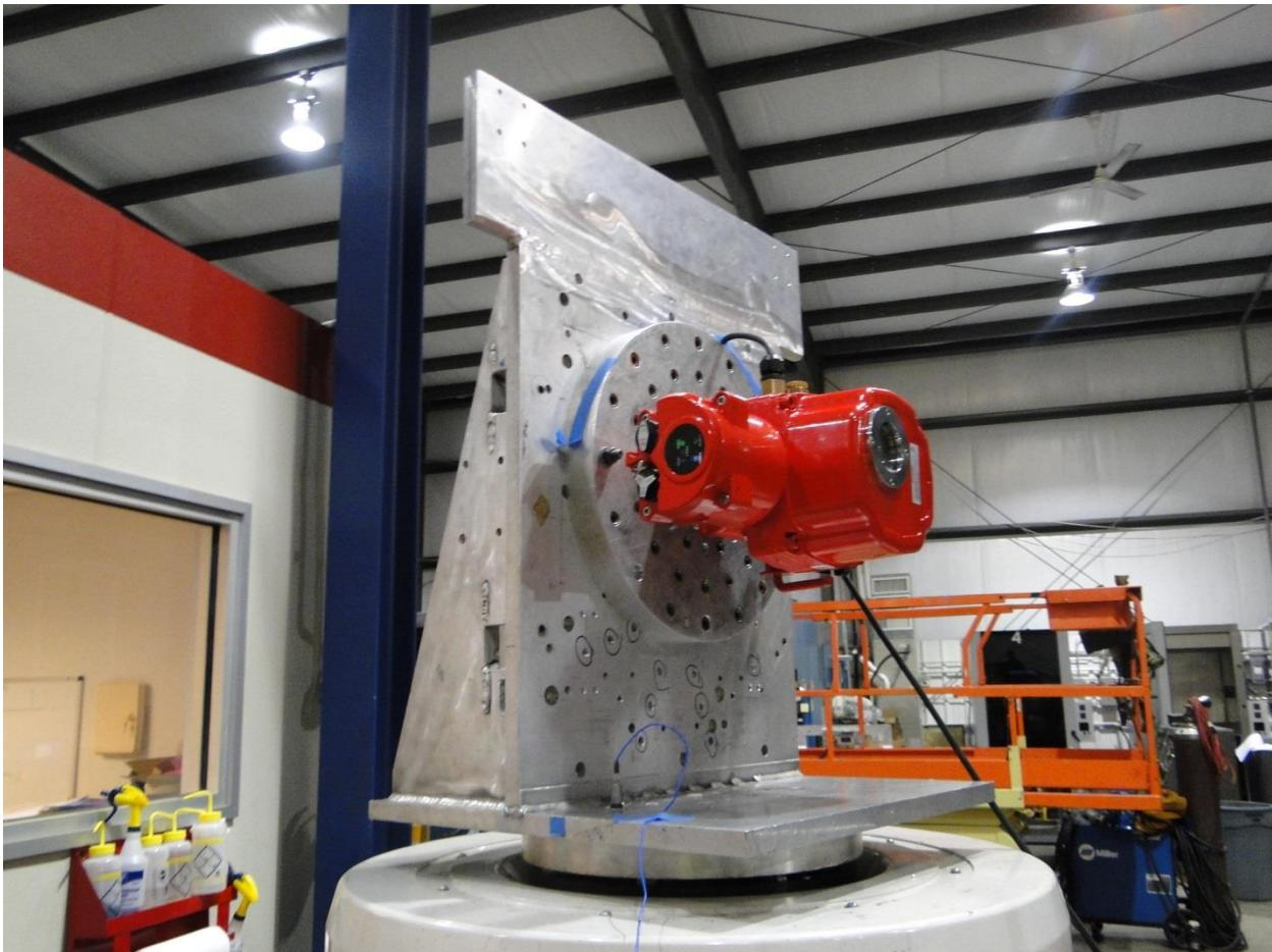
Photo 5.2.1-17 Longitudinal axis shock on WEM-4400
