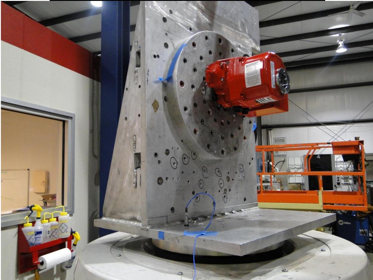
Photo 5.2.1-14 Transverse axis shock on WEM-690XD
