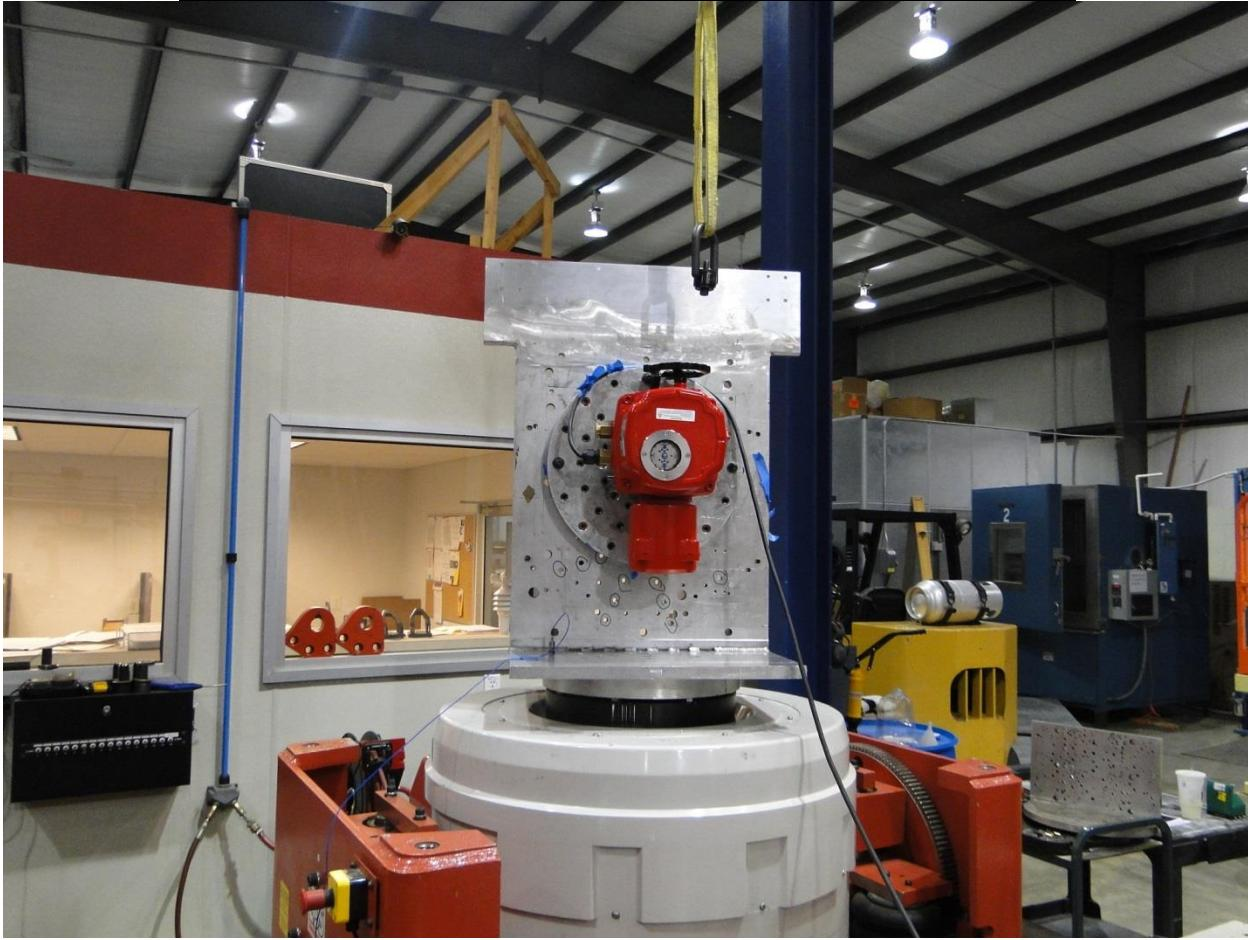
Photo 5.2.1-16 Longitudinal axis shock on WE-2640HB
