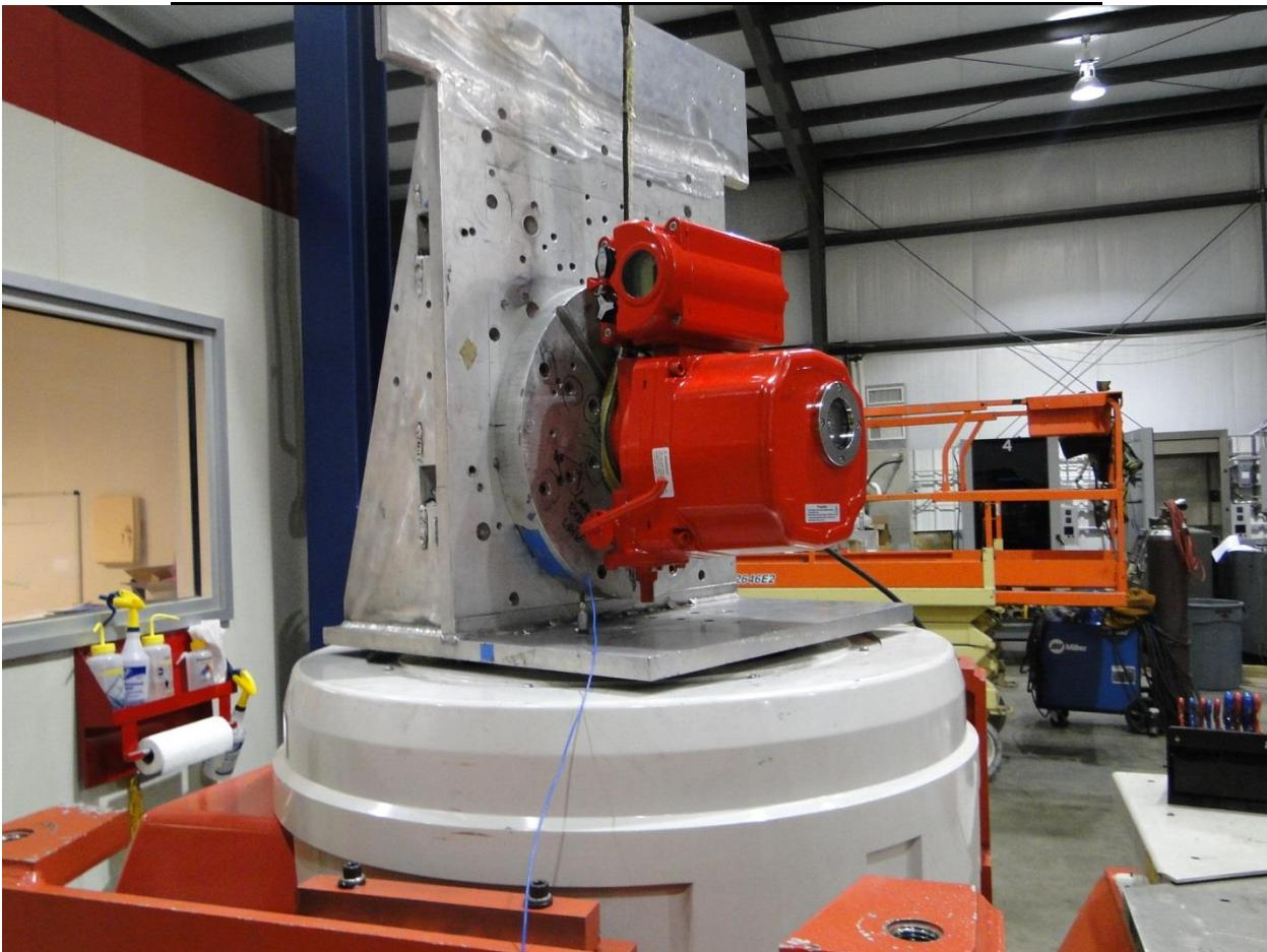
**Photo 5.2.1-11 Transverse axis shock on KEM-440XD**
