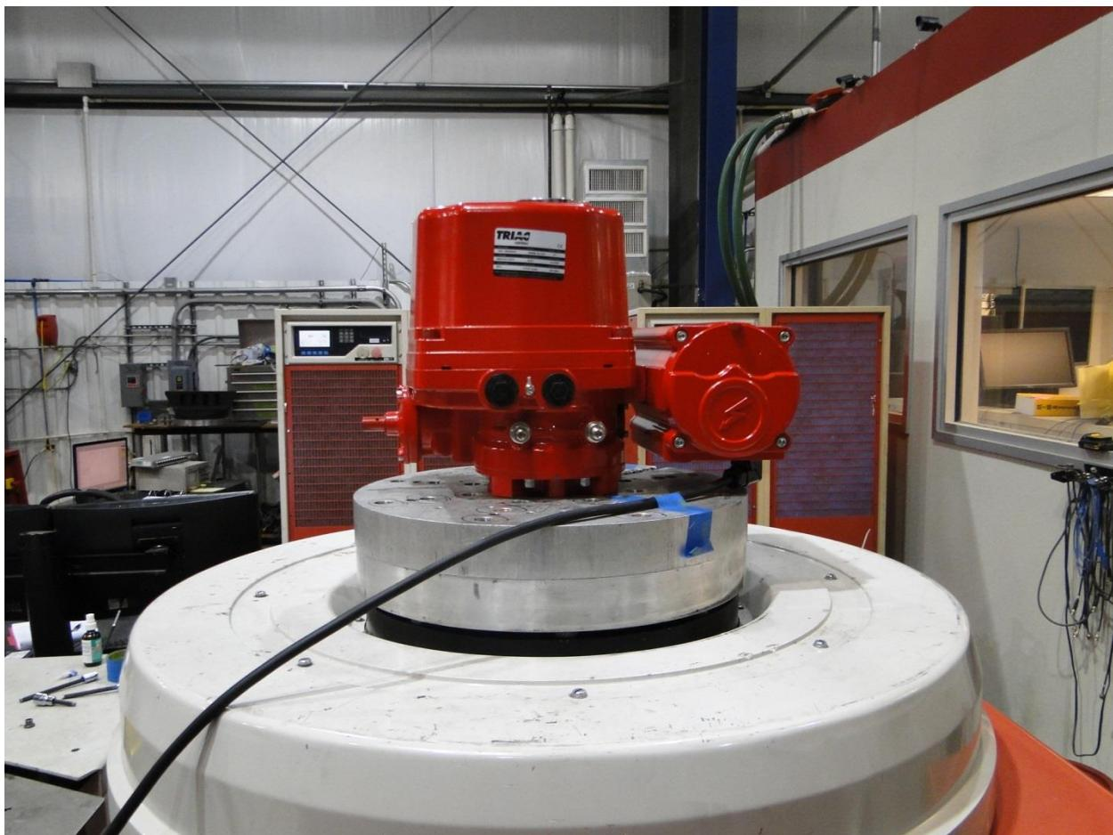
Photo 5.2.1-9 Longitudinal axis shock on WE-10500HB
