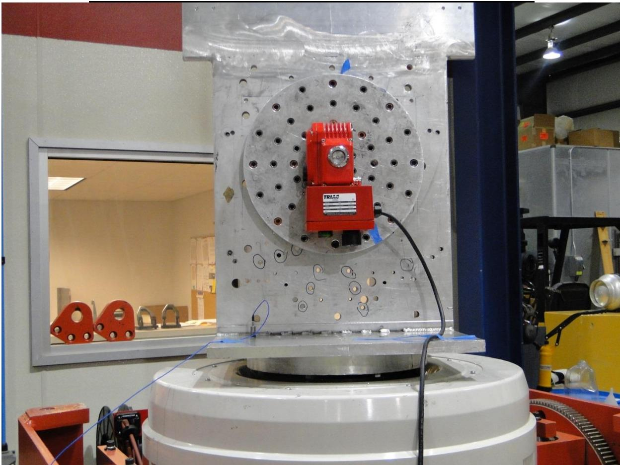
Photo 5.2.1-12 Longitudinal axis shock on KEM-440XD
