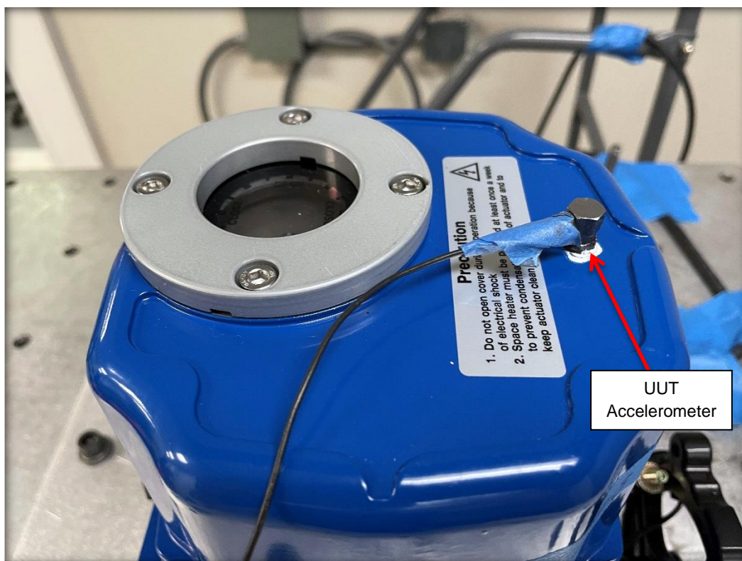
Figure 21: Detailed view of UUT accelerometer location for Z +ve axis testing – Type “SER” units
