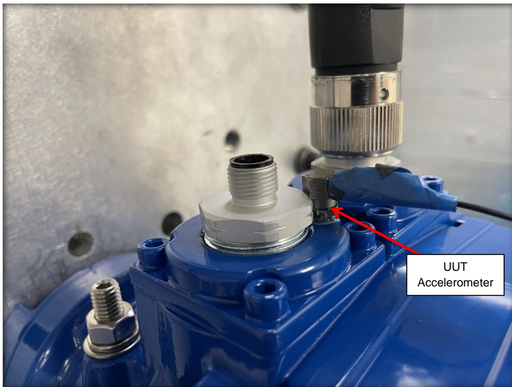
Figure 29: Detailed view of UUT accelerometer location for X +ve axis testing – Type “SER” units
